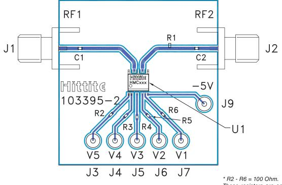
\* R2 - R6 = 100 Ohm. These resistors are optional and may be used to enhance decoupling of the RF path from the control inputs.
