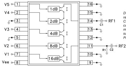
DC Blocking Capacitors C1 & C2 are required on RF1 & RF2. Choose C1 =  $C2 = 100 \text{ pF} \sim 0.1 \text{ uF}$  to allow lowest customer specific frequency to pass with minimal loss. R1= 5K Ohm is required to supply voltage to the circuit through either Pin 11 or Pin 14.
